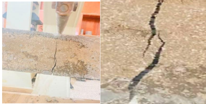
Figure 9. Reinforced mixes during flexural test.
